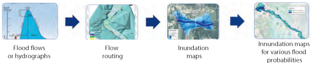
Figure 10. Inundation maps for the purpose of flood risk assessment (compiled by the author)
