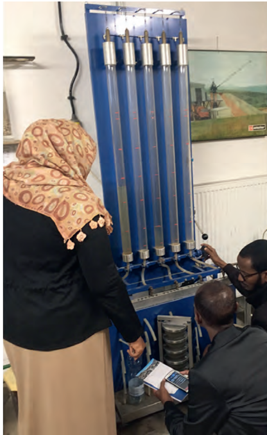
Figure 10. Atterberg-type settling device for PSD determination of fine sediments (photo taken by the author)
