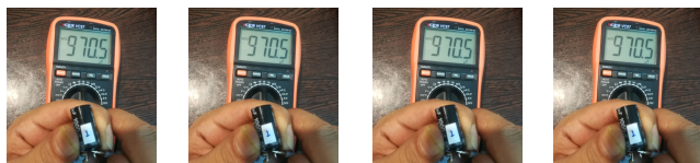
FIGURE 15. Measurement of the capacitance values of four capacitors.
