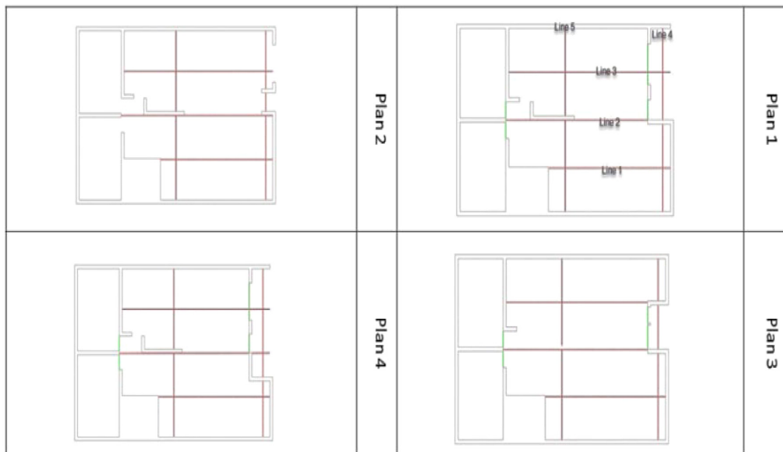
Fig. 14. Position of guidelines to explain airflow speed in plan 1 to 4.
