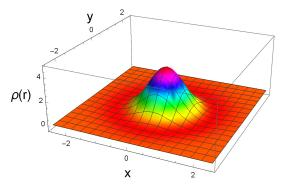
**Figure 9.** A 2D plot of the charge density as a function of the radius over time, where t = 1.0. Red color means zero charge density. The colors red, yellow, green, blue, and magenta, in that order, show the increasing charge density. The charge density and radius are understood in natural units.
