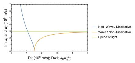
**Figure 6.** Dynamic transition between non-wave (dissipative) and wave-like (non-dissipative) propagation. The critical transition point is at  $Dk_0 = c/2$ . The diffusivity parameter is D = 1. The phase velocity of  $w_f$  of the wave-like propagation is always less than the speed of light.
