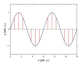
**Figure 1.** Mechanical Klein–Gordon wave propagation, with a string of density  $\rho$  stretched by a force F. The red lines demonstrate the attractive linear force field. This force field is proportional to the vertical displacement  $-k_a y$ . This is the "extra" interaction compared with the usual transverse wave.
