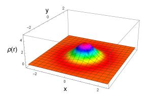
**Figure 8.** A 2D plot of the charge density as a function of the radius over time, where t = 0.7. Red color means zero charge density. The colors red, yellow, green, blue, and magenta, in that order, show the increasing charge density. The charge density and radius are understood in natural units.
