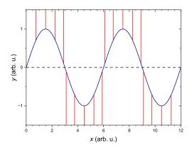
**Figure 2.** Mechanical Klein–Gordon wave propagation, with a string of a density  $\rho$  stretched by a force F. The red lines demonstrate the repulsive linear force field. This force is proportional to the vertical displacement  $k_a y$ .
