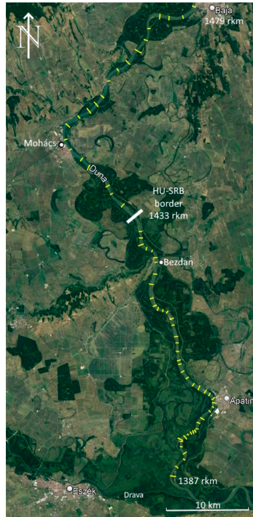
Figure 2. Investigated river reach with indicated positions of surveillance cross-sections (yellow marks) on the Hungarian and Serbian sides. The white line presents the border. The average distance between the cross-sections in Hungary is approximately 2000 m and in Serbia 1000 m.
