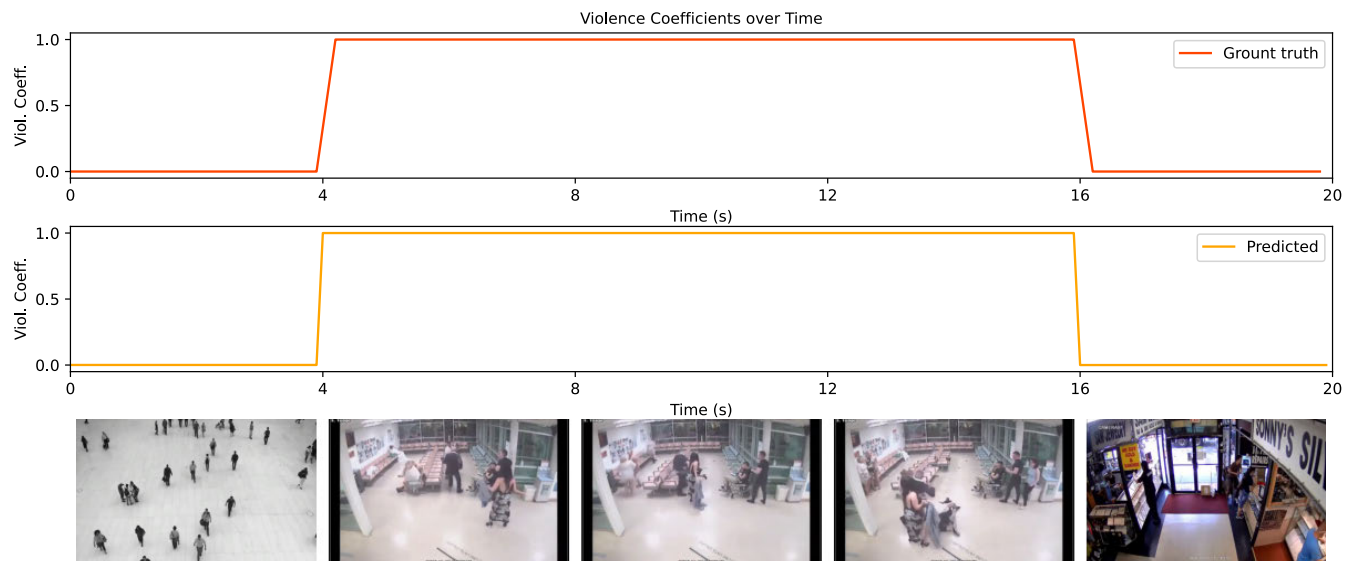
FIGURE 19. Results of our standalone system using FT model on a video compiled from 3 random videos of Smart-City CCTV Violence Detection Dataset, one violent and two non-violent videos concatenated in such a way that the violent video is placed in between two non-violent videos. Row 1: Ground truth of violence coefficients over time. Row 2: Predicted violence coefficients on 4-second video segments. Row 3: Keyframes extracted from the video.
