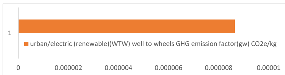
Figure 19. TIPI for environment aspect, GHG emission factor in € CO 2 e per passenger-km for electric (renewable sourced energy) train.
