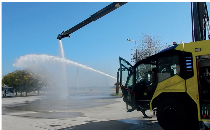
Picture 3: An airport fire engine with working monitors
