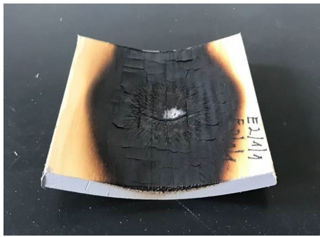
Fig. 7 Concave deformation of Scots pine
