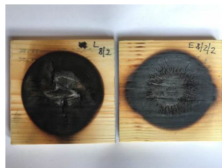
Fig. 6 Visible cracking of the test samples
