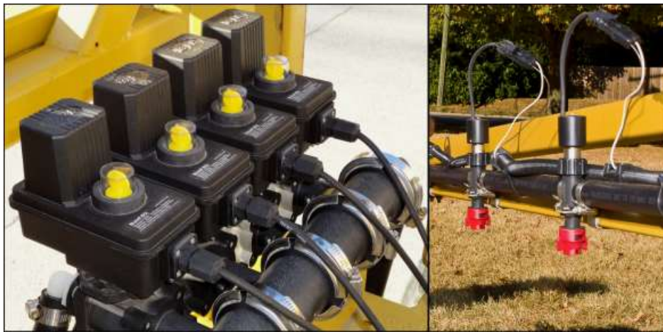
Fig.72. Boom section valves (left) and individual nozzle valves (right) are used with automatic boom section control systems (source [188]).
