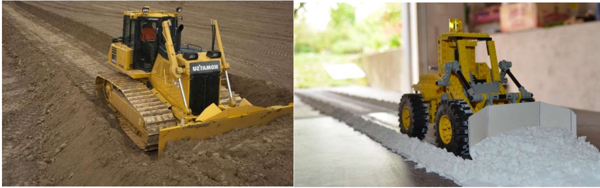
Fig.38. Windrows happening on the side of blade, prepared by the author.
