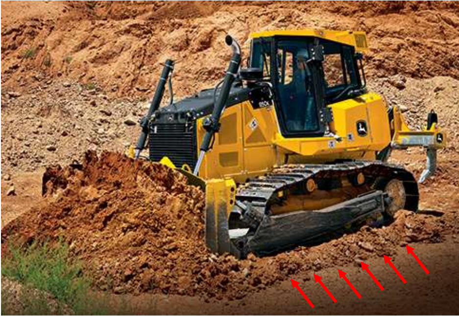
Fig.23. Windrows on the side of a dozer after it filled to capacity, prepared by the author.
