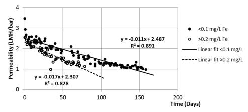
**Figure 7.** Relationship between permeability with 100  $\mu$ g/L and 200  $\mu$ g/L dissolved iron and time (LMH = L·m<sup>-2</sup>·h<sup>-1</sup>).
