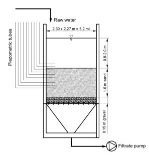
Figure 1. Slow sand filter layout.
