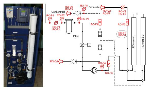
**Figure 2.** Small scale reverse osmosis (RO) unit (measurement points: F = flowrate; C = conductivity; P = pressure; Q = sampling; T = temperature; V = volume).
