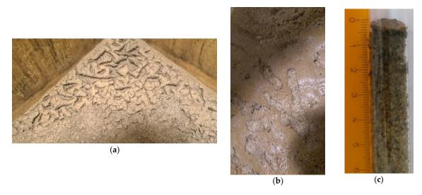
**Figure 5.** Clogged layer at the porous media–water boundary. (**a**) Dried state; (**b**) wet state; (**c**) approximate thickness of 2–3 mm.
