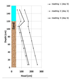
Figure 3. Measured pressure distribution in filter.
