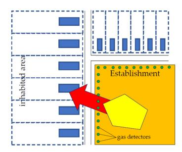
Figure 2. Installation of gas detectors (schematic figure). Source: own research.
