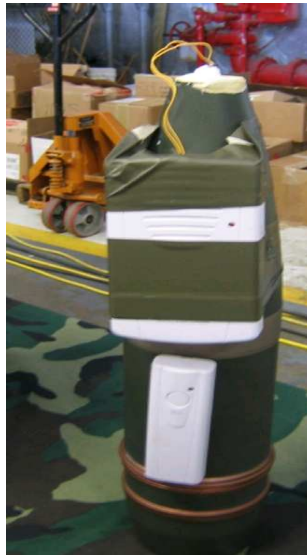
Figure 8. Wireless door bell as a controller for RCIED. [12]
