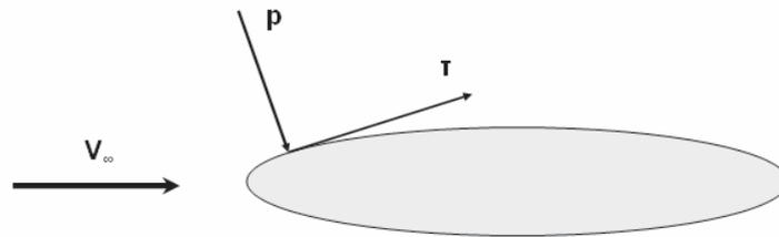
Figure 1. The pressure ( $p$ ) and shear stress ( $\tau$ ) on the surface of object located in the freestream moving with velocity  $V_\infty$  (after ANDERSON, 2001).
