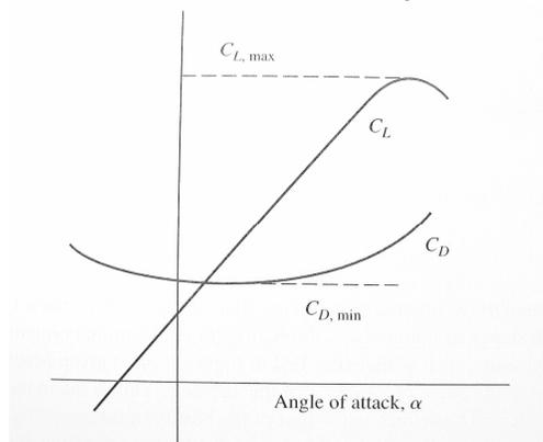
Figure 3. Relationship between lift and drag coefficients and angle of attack ( $\alpha$ ). The maximum lift ( $C_{L,max}$ ) and minimum drag coefficients ( $C_{D,min}$ ) are signed (after ANDERSON, 2001).
