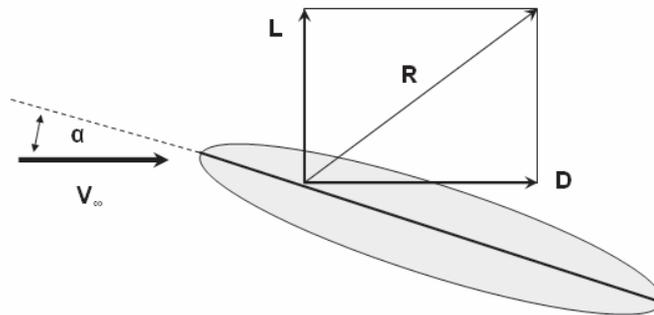
Figure 2. The resultant aerodynamic force and its components: lift ( $L$ ) and drag ( $D$ ) force.  $\alpha$  is the angle of attack and  $V_\infty$  is the freestream velocity (after ANDERSON, 2001).
