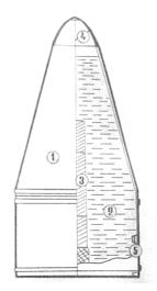
Figure 2. Russian chemical warhead for tactical missile. 1. Body, 2. chemical agent, 3.explosive charge, 4. fuze, 5. filling plug It contained 555 kg VX
