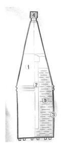
Figure 3. Chemical warhead of tactical missile . 1. Body, 2. explosive charge, 3. filling plug, 4. fuze, 5. chemical agent. The warheads contained 216 kg VX
