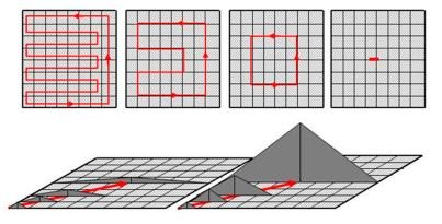
**Figure 2.** If camera view angle increases or flight altitude is higher flight path moves to the center of the observed area. In this case, other conditions such as the edge of the area remain unchanged. Source: author.
