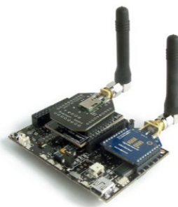
4.2. ábra: Libelium Wasp mote Expansion Radio Board
