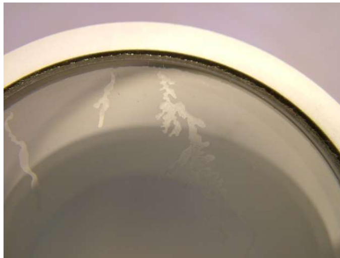
Figure 23. NaI(Tl) crystal disunion example. Source: [62]
