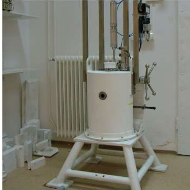
Figure 31. Irradiator with multiple source positions. Source: [3]
