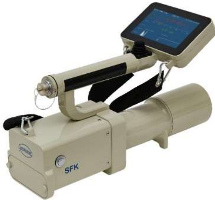
Figure 50. SFK search and isotope identification unit Source: [3]
