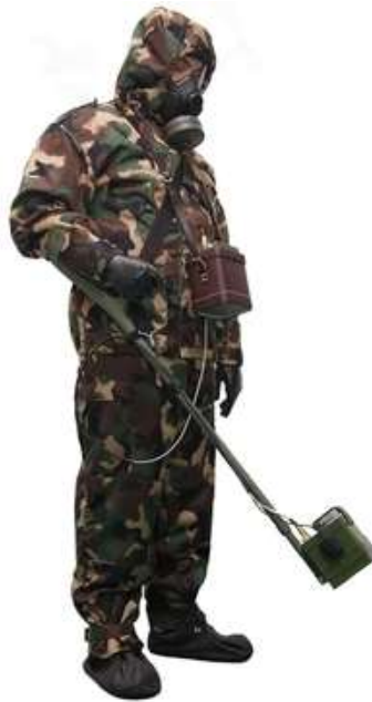
Figure 56. IH-295 surface contamination monitor in operation.
