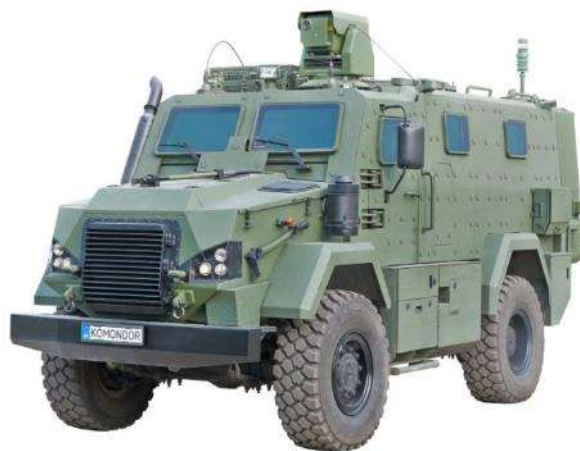
Figure 7. RDO-3221 ABV Komondor CBRN reconnaissance vehicle Source: [3]
