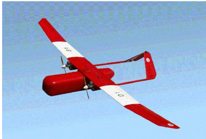
Figure 13: SAS – type, a long range, multiple purpose UAV with 2 IC piston engines (Designed by Electronic Warfare Department of MZNDU)
