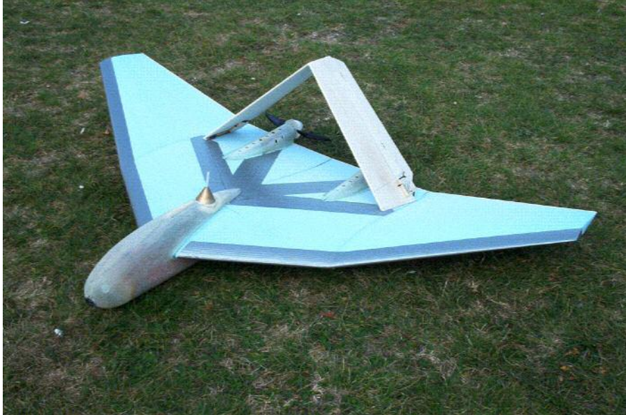
Figure 18: DELTA close reconnaissance UAV with electric driving pitch (Designed by Electronic Warfare Department of MZNDU)
