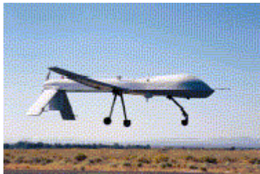
Figure 14: PREDATOR (Tier-2) operational reconnaissance UAV with IC piston engine driving rear pitch
