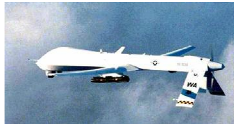
Figure 14: PREDATOR (Tier-2) operational reconnaissance UAV with IC piston engine driving rear pitch
