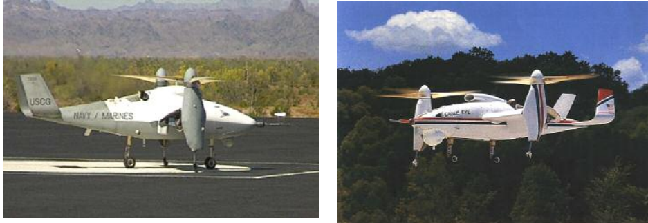
Figure 15: EAGLE EYE STOL multi-purpose reconnaissance UAV with GT engine driving pitch
