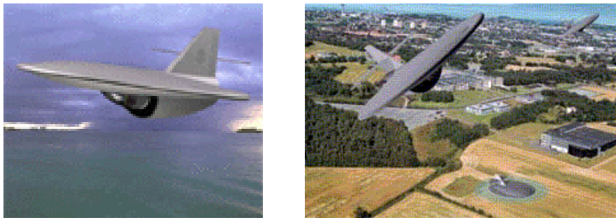
Figure 17: The Norwegian SRC UAV: single rear jet engine below it-and a conventional tail plane above
