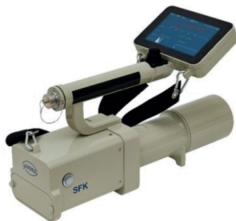
Figure 5. SFK search and isotope identification unit
