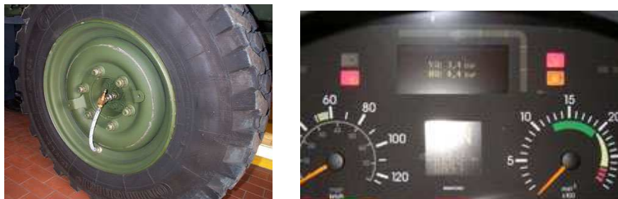
Fig.: 4.8. The indication of the tyre filling valve and tyre pressure values
