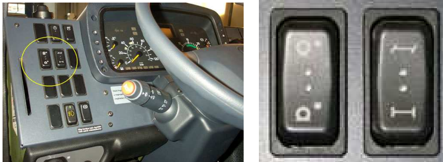
Fig.: 4.7. Pressure regulator switches
