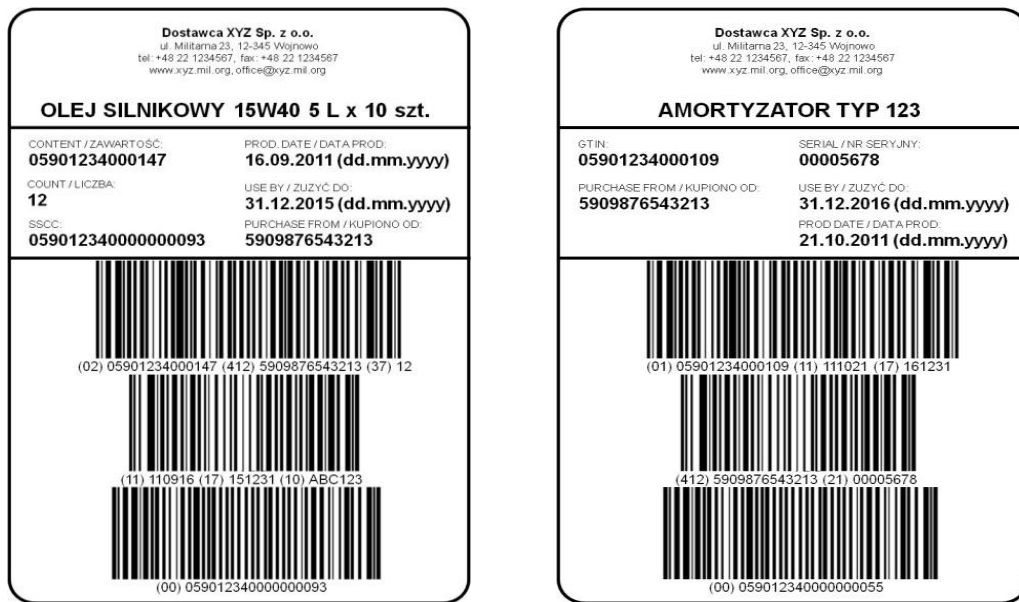
Pict. 9 - Examples of GS1 logistics labels being used in the Polish military sector for logistic items (for all assortment groups). The range of information encoded in the barcode depends on the content of logistic unit.
