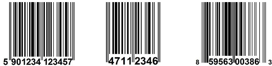
Pict. 7 - Examples of GSI barcode symbols using in the Polish military sector for retail trade items (for all assortment groups): EAN-13, EAN-8, UPC-A
