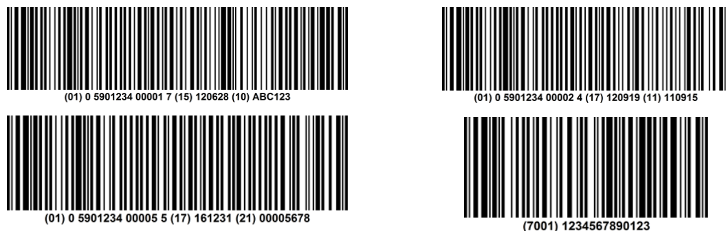
Pict. 8 - Examples of GS1-128 barcode symbols using in Polish military sector for non-retail trade items (for all assortment group). The additional information encoded in barcode depends on the specific assortment groups.
