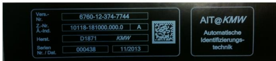
Pict. 8 - Exemplary type plate of KMW including GS1 DataMatrix
