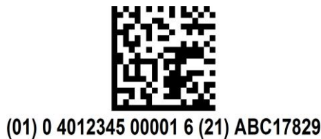
Pict. 7 - Exemplary GS1 DataMatrix with GTIN and serial number
