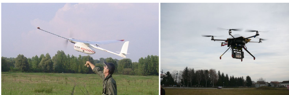
Figure 4. Launch of fix wing drone (Fenix) for fire reconnaissance before starting intervention. Rotary wings drone (Bee) hovering at forest fire. Source: 6DOF (Croatia) and R-Fire Ltd. (Hungary)
