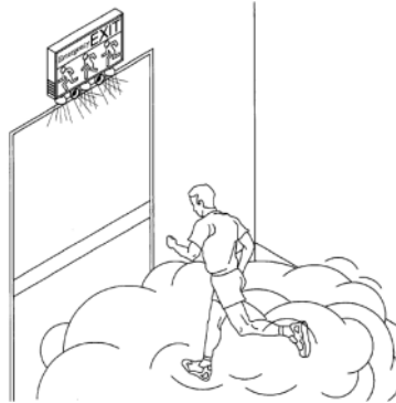
Figure 2: dynamic emergency escape indicator [8]
