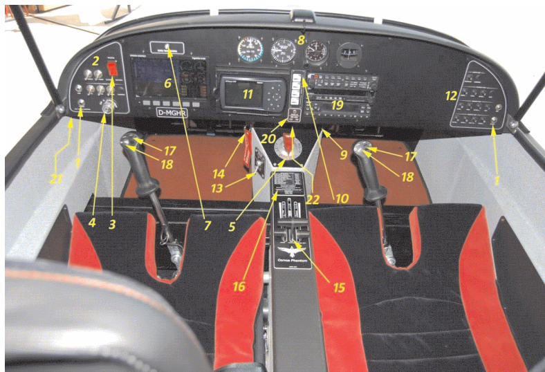
Fig. 3. Integrated on-board system Corvus CA-21 Phantom cockpit
