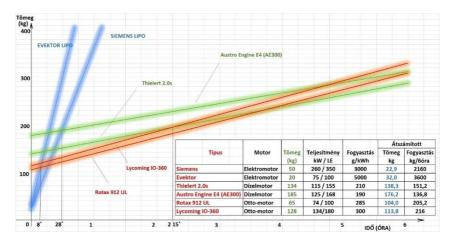
Diagram of weight necessary for a given flight time in cases of petrol, diesel and electric engines
