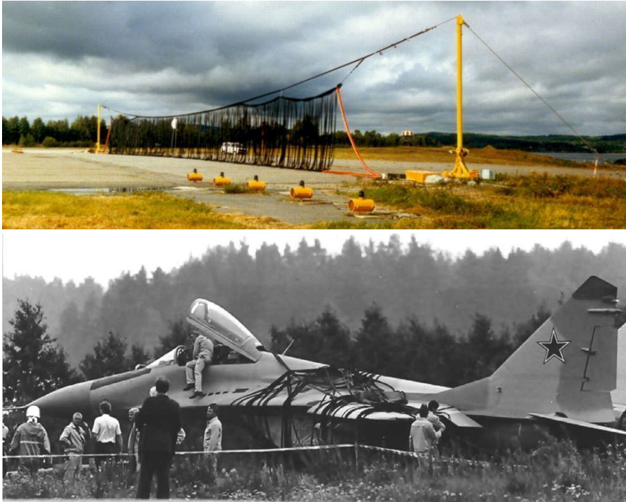
Fig. 3. UOTILA-24 Barrier Net installed at Kuopio Airport in Finland
