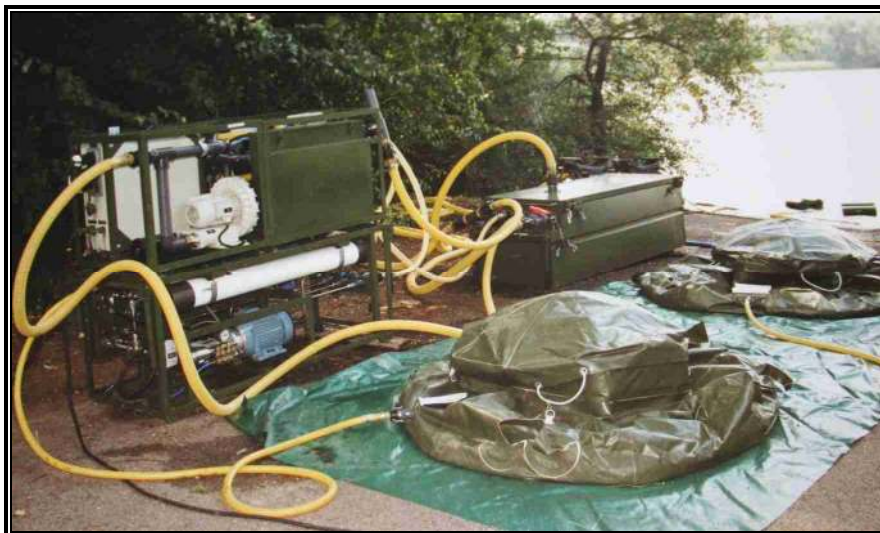
Figure 2: ZENON Mobile Potable Water Treatment System 2
