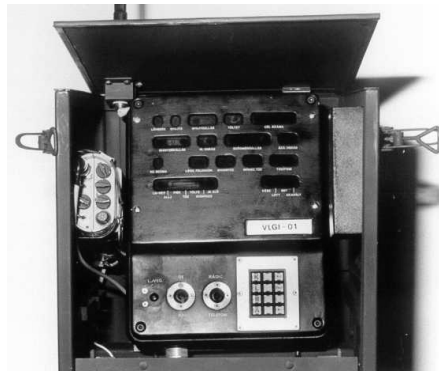
Figure 2. Gun Display Unit of the ARPAD system for towed battalions (Photo: MoD Institute of Military Technology)
