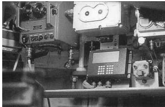
Figure 5. Interface and control unit of position data transformer of the ARPAD M system built in the battalion commander vehicle turret (Photo: MMG AM Co. Ltd.)
