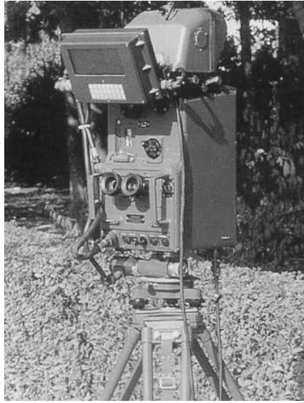
Figure 4. Digitised external laser rangefinder of the ARPAD M system (Photo: MMG AM Co. Ltd.)
