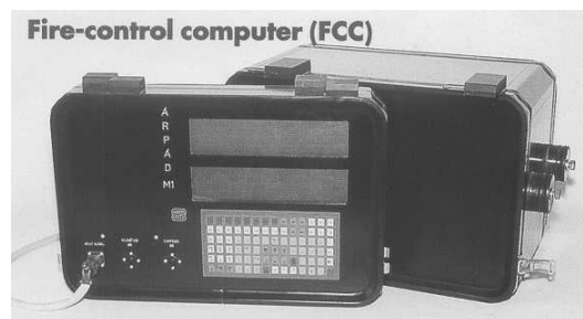
Figure 7. The new Unified Command Post Computer of the ARPAD M1 fire control system (Photo: MMG AM Co. Ltd.)
