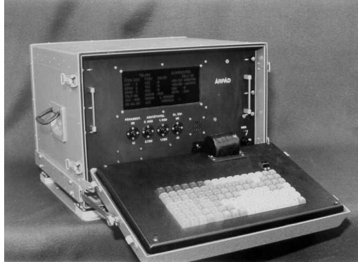
Figure 1. Command Post Microcomputer of the ARPAD system with gas plasma display (Photo: MoD Institute of Military Technology)
