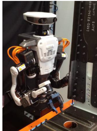
Figure 40. Dual Arm concept 'Next Age' in an aeronautics assembly operation [40]
