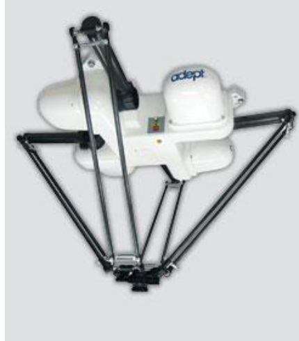
Figure 4. Example of a 4-axis delta robot [4]
