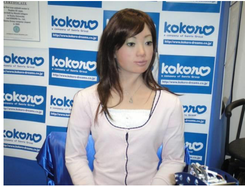
Figure 28. 8-axis android receptionist with integrated vision from Kokoro Inc. Japan [28]
