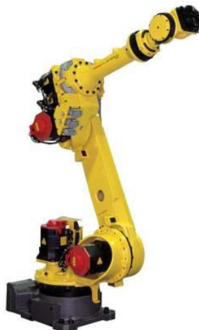
Figure 3. Example of a 6 axis articulated robot [3]
