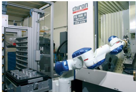
Figure 35. 7-axis articulated robot by Motoman loading a machine center [35]
